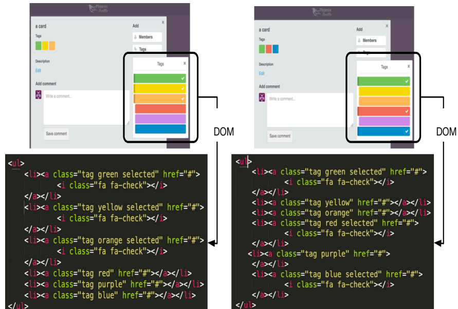
Figure 3.13: Undetected near-duplicate fragments in phoenix
